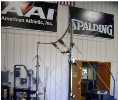
far, it's all good, but when that rail flexes, the distance from end to end must decrease because the bar does not have any end to end elasticity. Therefore, in order for the bard to flex, and the ends to come in, the uprights (vertical supports) must move in, forward, or back depending on which direction the bar is flexing. The uprights are anchored by steel cables which also do not stretch so they just transfer the force to the tie down that is connected into the floor anchor.
